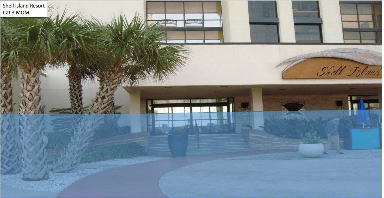
Figure 14: Category 3 Maximum of Maximum Storm Surge Inundation (Water Height Represented by Pale Blue Line) at the Shell Island Hotel in Wrightsville Beach, North Carolina (FEMA 2016)
