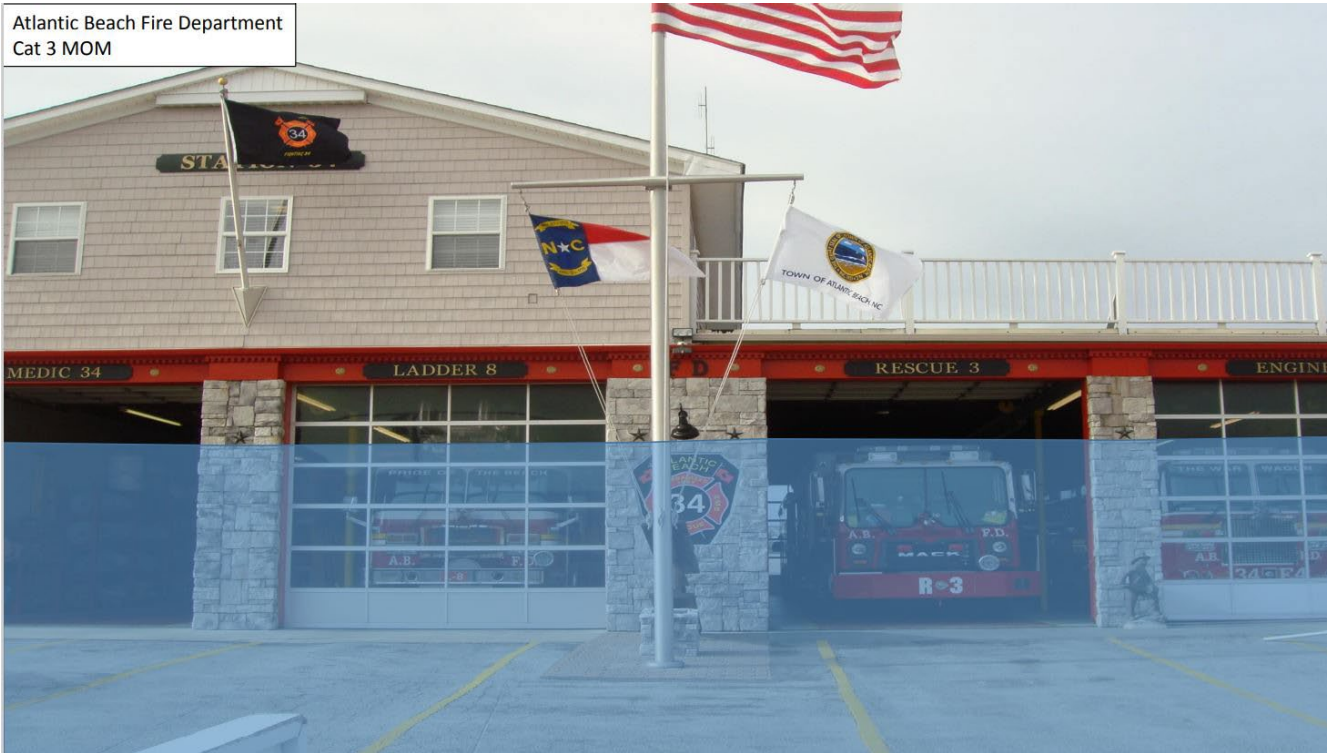
Figure 12: Category 3 Maximum of Maximum Storm Surge Inundation (Water Height represented by Pale Blue Line) at the Atlantic Beach Fire Department, Carteret County (FEMA 2016)
