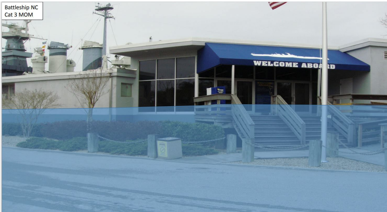
Figure 16: Category 3 Maximum of Maximum Storm Surge Inundation (Water Height Represented by Pale Blue Line) at the USS North Carolina Battleship Memorial on the Cape Fear River (FEMA 2016)
